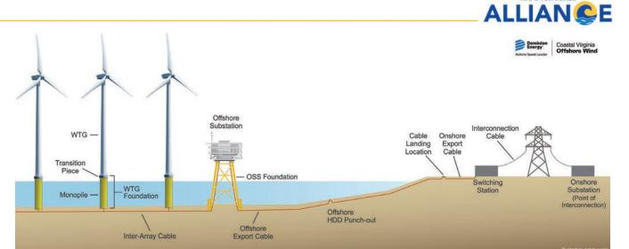
Offshore wind farms require substations and hundreds of miles of submarine transmission cable. Source: Dominion Energy
